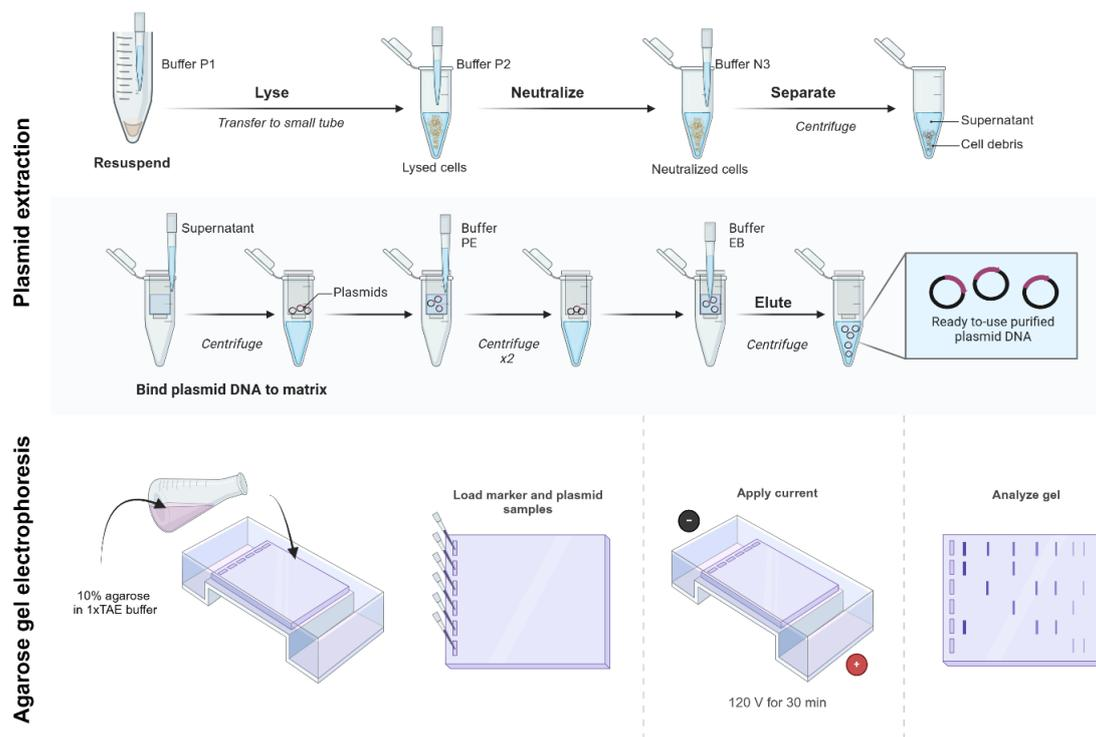
**Figure 7: Plasmid DNA extraction and agarose gel electrophoresis protocol.** The scheme was created with BioRender. V – volt, min - minutes
