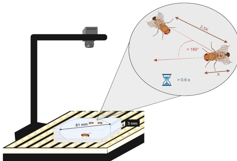
**Figure 16: Video recording station for SIN experiment.** Criteria for interaction between flies are marked on the scheme. The scheme was created with BioRender. mm – millimeters, s – seconds, ° - degree.
